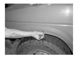
3. Remove the arch and carefully cut the wing just a fraction above your marked line. Cutting the wing is easily done with a 4" angle grinder with a metal cutting disc, make sure you wear goggles for this.
